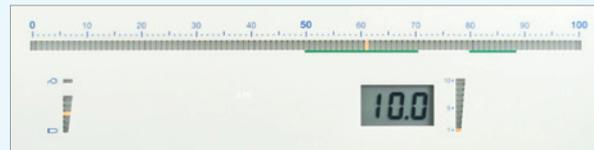
Measurement can be taken automatically, which shows the highest value and the indicator drop. If you wish to work like with a standard device with analogue indicator just switch to manual mode.
