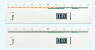
Measurement can be taken automatically, which shows the highest value and the indicator drop. If you wish to work like with a standard device with analogue indicator just switch to manual mode.
