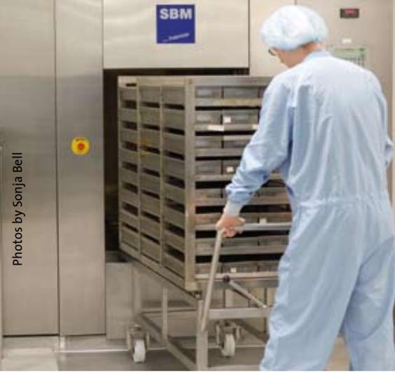
*Manual loading of ampoules into a sterilizer*
