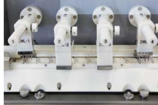
discharged from the labeler, it is monitored by another sensor that confirms the presence of a label. This equipment can label about 330,000 ampoules per day. After labeling, the finished Traumeel ampoules are spot-checked for correctly applied and printed labels.
